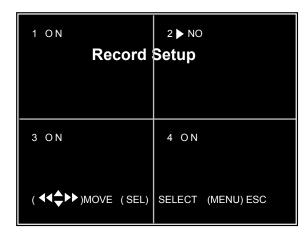
The Record Setup sub-menu allows you to choose which channels (cameras) will record.
